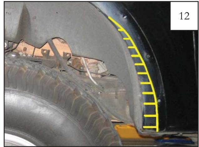
At 1-1/2" intervals, make horizontal lines from fender lip to line drawn in Step 11. These lines will be cut later, forming tabs to be hammered in.
