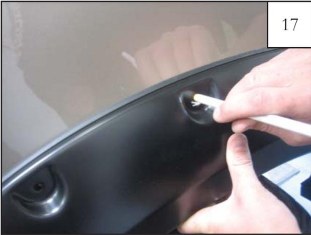
Position fender flare on fender. Verify that parts fit and no additional cutting is needed. Maintaining part position, mark the hole locations in the fender using the pocket holes in the flare as guide (8 places).
