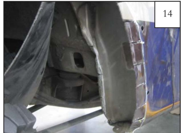
Using a hammer, pound the pinch weld flat up to the 9" mark made in Step 13. Using a reciprocating saw or cut-off wheel, cut horizontal lines made in Step 12.
