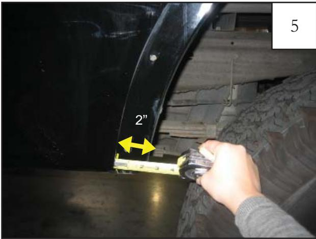
At FRONT of wheel well, use a tape measure and a grease pencil to mark a line 2" toward front of vehicle from fender lip (at bottom edge).
