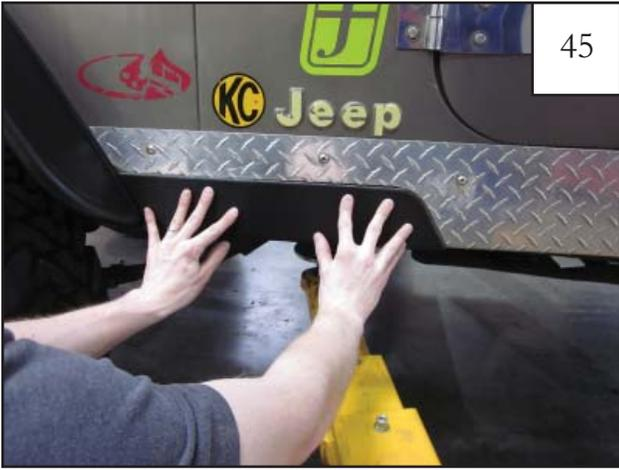
After the red liner is removed, *firmly* press the rocker panel against the vehicle for 10 seconds to adhere the tape to the vehicle surface. The vehicle surface temperature must be between 65-110° F for proper adhesion. Allow 24 hours for full adhesion.
