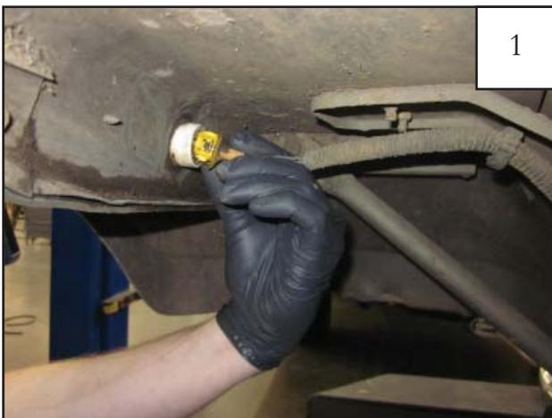
Unplug the factory installed side marker lamp by twisting the bulb housing in a counterclockwise direction. This is located at the front of the factory flare on the backside in the wheel well.
