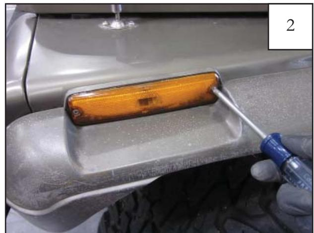
Remove the factory installed side marker lamp using a #2 Phillips head screw driver.
