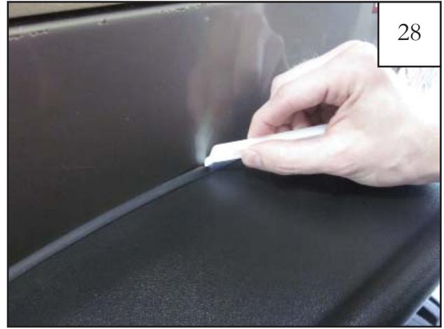
Use the hooked end of the Edge Trim Tool (ET1-0002) to check for full adhesion. Do this by sliding it along the top of the edge trim to visually verify that the tape is adhered to the vehicle surface. Repeat Step 27 if the tape is not fully adhered to the vehicle surface.
