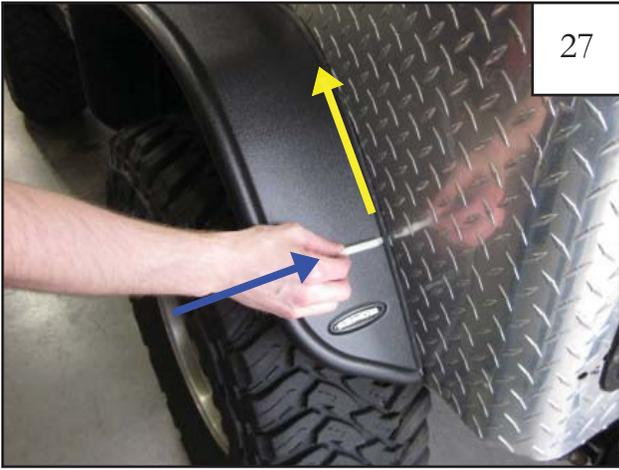
Starting at one end, use the flat edge of the supplied Edge Trim Tool (ET1-0002) to further adhere the edge trim to the vehicle surface. Slide the tool along the edge trim while pressing it in toward the vehicle surface.
