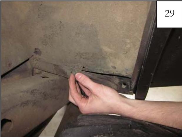
Using fasteners removed in Step 2, reinstall the rear wheel well skirting.
