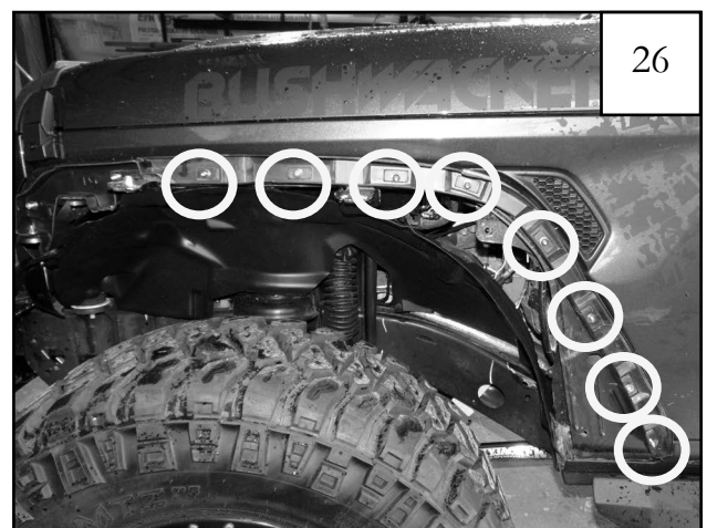
Step 3 Secure inner piece D2 with allen bolts and washers using the same procedure described in Step 24 and 25.
