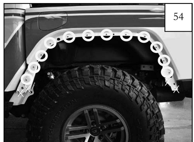
Install (12) rivnuts in rear fender area using the same procedure as Steps 13 thru 17. Test fit inner pieces LR3, LR2, and LR1 (Front to back). *NOTE: The "X" above indicates a hole that is not used.*
