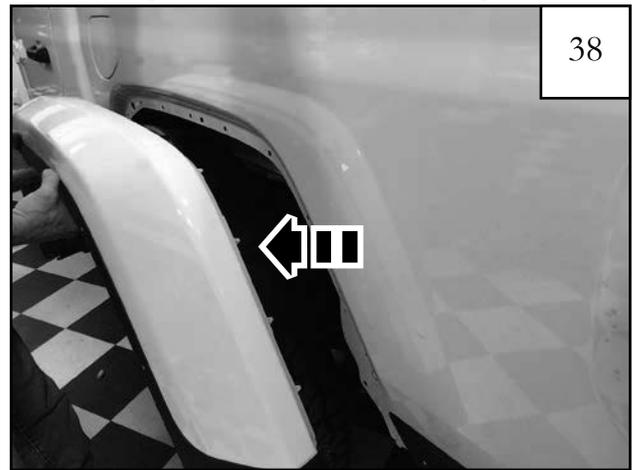
Starting at front of flare, pull *firmly* to release flare and splash shield from fender, working your way to the back. You will hear popping noises as clips release. It is okay if clips break, they will be discarded. Discard fender and fender liner.
