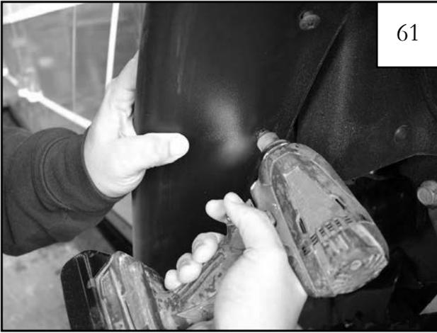
**AFTER ALL SCREWS HAVE BEEN STARTED,** tighten the screws by *firmly* pressing the flare toward the vehicle *while* tightening.
