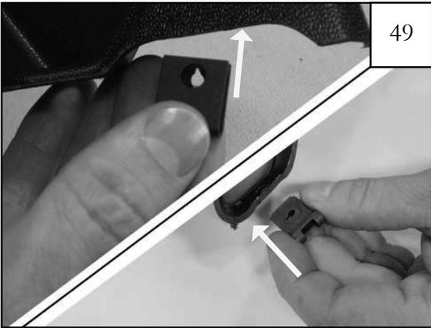
Install a CL1-0022 U-clip at each clip location on the inner pieces, centering them on the predrilled holes with threaded portion on inside. (9 locations) *NOTE: Clips may slide out of place. Try pinching the metal tightly onto the inner piece with pliers.*
