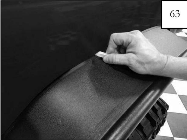
Use the hooked end of the edge trim tool to check for proper placement of rubber gasket. Do this by sliding it along the top of the edge trim and visually verify that the wiper is positioned correctly.
