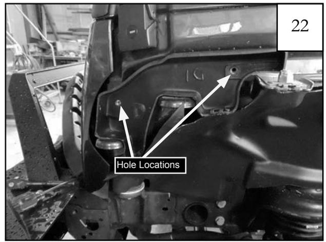
Secure inner piece D1 (and P1 for passenger side installation) to the sheet metal using the following **3 Steps: Step 1** Position inner piece on fender by aligning holes with previously installed rivnuts.
