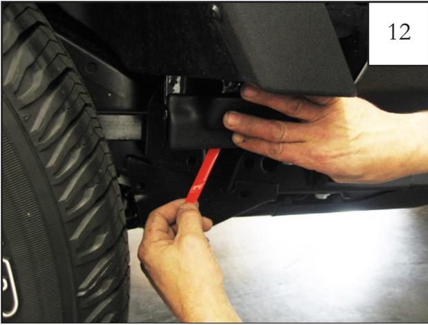
Toward the rear of the vehicle, pull 1/2" tape liner tab 6. Press firmly on the part following tape liner removal. *NOTE: Refer to step 1 for additional tape tab identification.*
