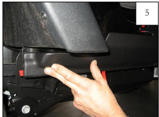
Place part on vehicle, making sure to line up edges of part with edges of vehicle. Ensure that all tape tabs are accessible. **NOTE: Refer to step 1 for placement of certain tabs.**
