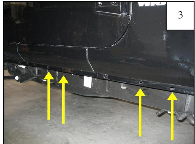
Locate the four factory holes in the rocker.
