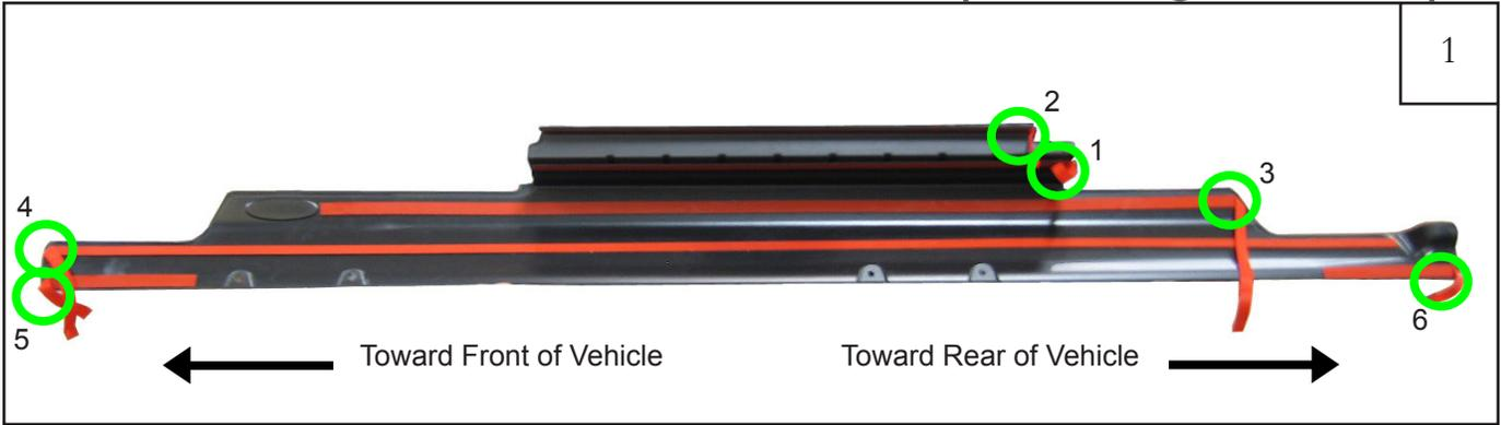
Using a marker, number the tape tabs as shown:
