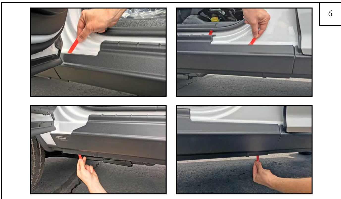
Set part in place on vehicle. Remove all red tape liners. Apply **FIRM** pressure to mounting locations to affix to truck.
