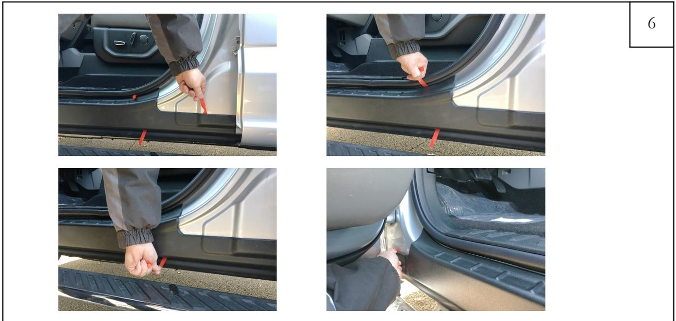
Set part in place on vehicle. Remove all red tape liners. Apply **FIRM** pressure to mounting locations to affix to truck.
