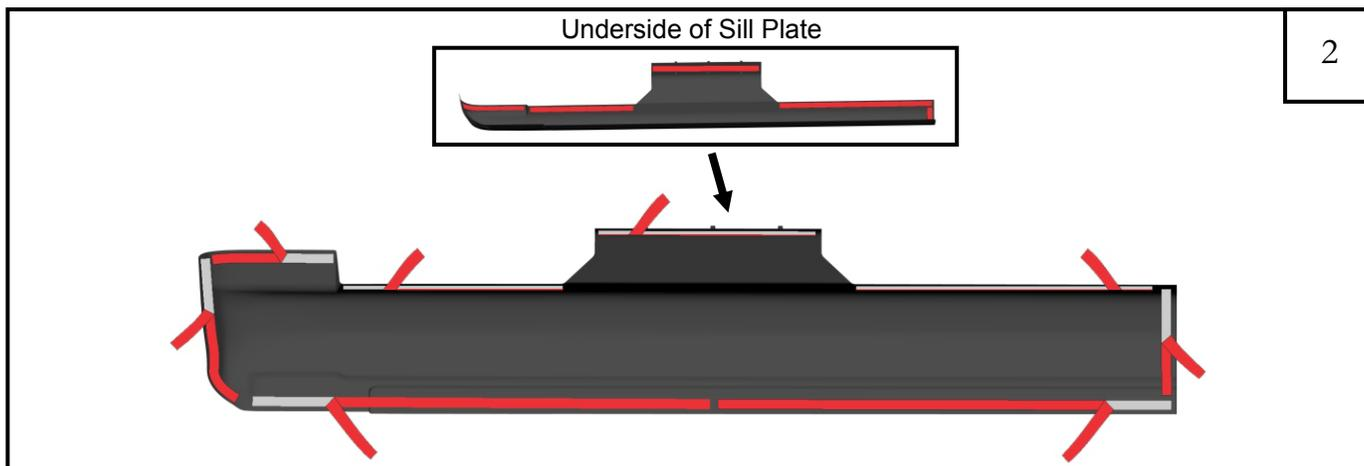
Open vehicle doors. Clean all dirt and debris from vehicle door sills and rocker panel. Use supplied alcohol wipes where part will attach.
