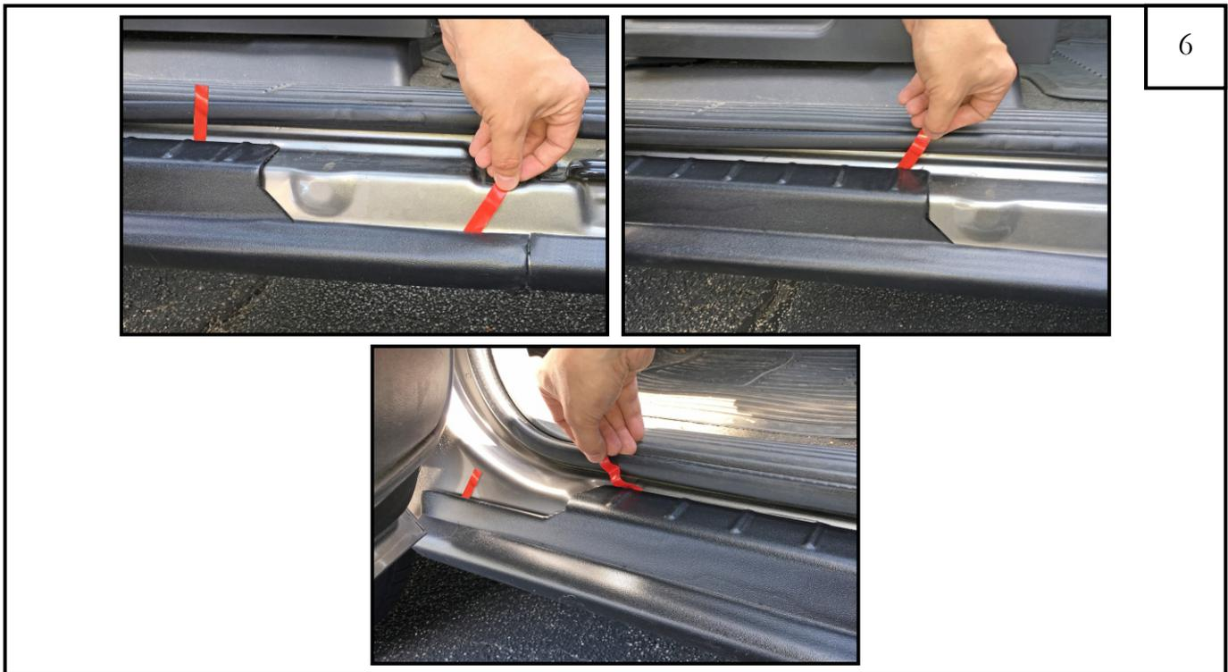
Set part in place on vehicle. Remove all red tape liners. Do not forget tape liners on bottom of part. Apply **FIRM** pressure to mounting locations to affix to truck.
