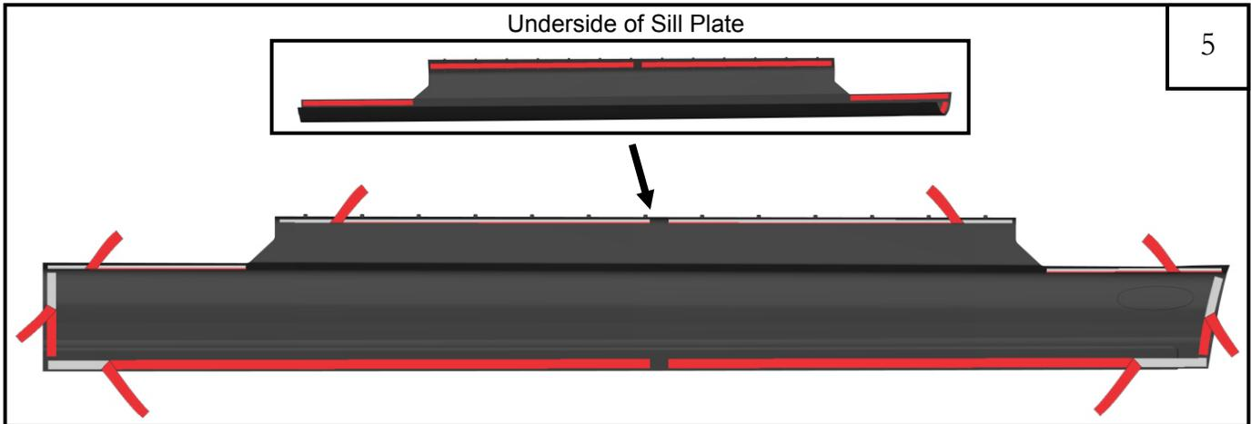
Peel back roughly 3" of red tape from the pieces of tape on the back side of the front part. Make sure red tape liner will be accessible when part is attached to truck.
