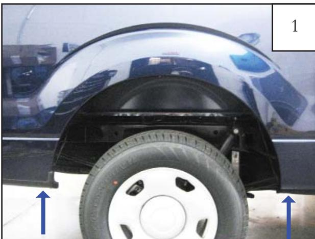
Remove two factory bolts with a 10mm socket wrench and discard. (Note: New hardware is supplied, see Step 6)
