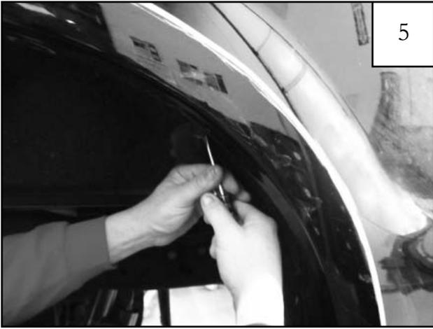
Using a pry tool, remove two factory installed tuftlocs from splash guard
