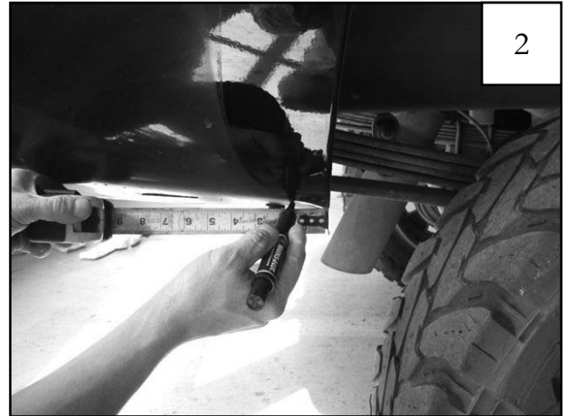
2 At each end of the wheel well opening, measure in 1.5" and mark.
