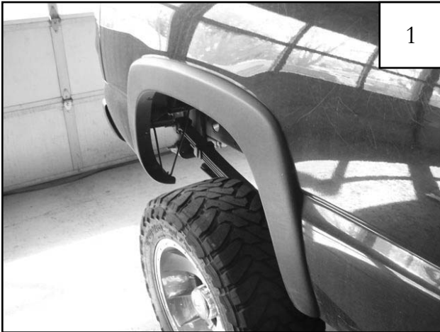
1 Remove factory flare using a flat blade screwdriver to pry up the head of the fastener.
