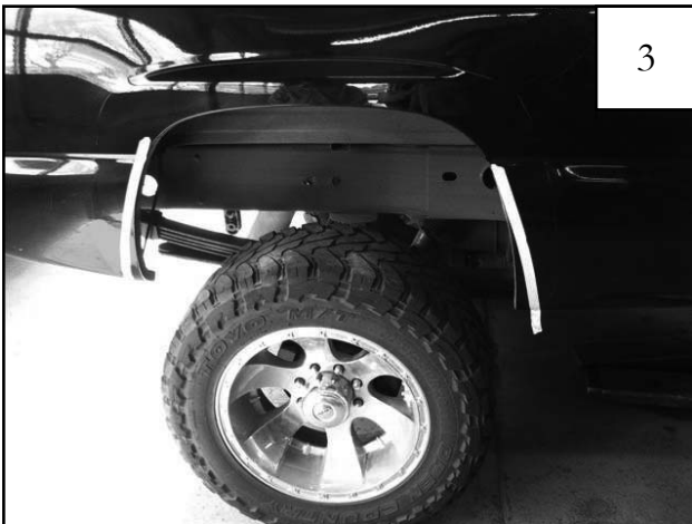
3 From each mark, run a tapeline vertically observing fender well curve to intersect with the tangent of the wheel well opening. (Middle of the bodyline or bottom edge of the tub.)
