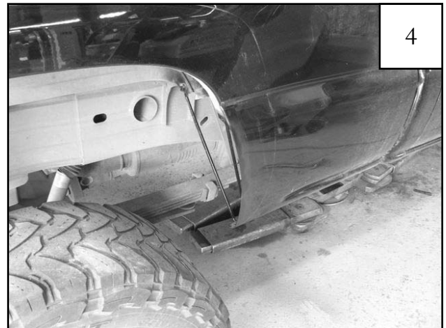
4 Using a cut off wheel, cut along inside of tapelines. Deburr edges and seal with primer or undercoating.
