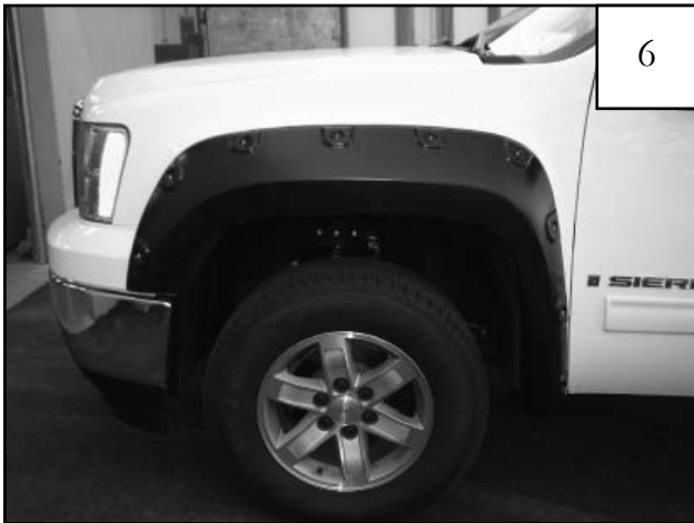
Completed front flare installation.
