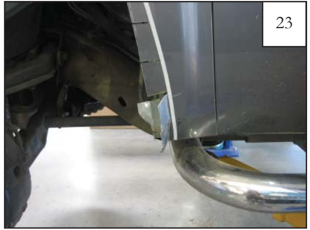
Bend lowest two metal tabs outward.
