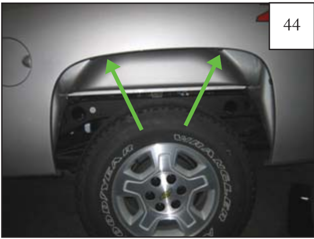
Slide a supplied Clip (CL1-0022) over top two tabs. Clips may need to be adjusted to align with holes in flare.
