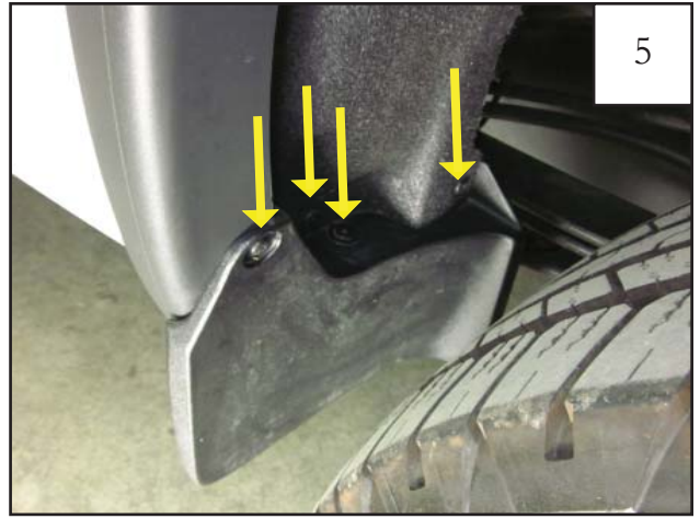
Using a T-15 Torx bit, remove the 4 factory screws from the plastic wheel well piece and remove.
