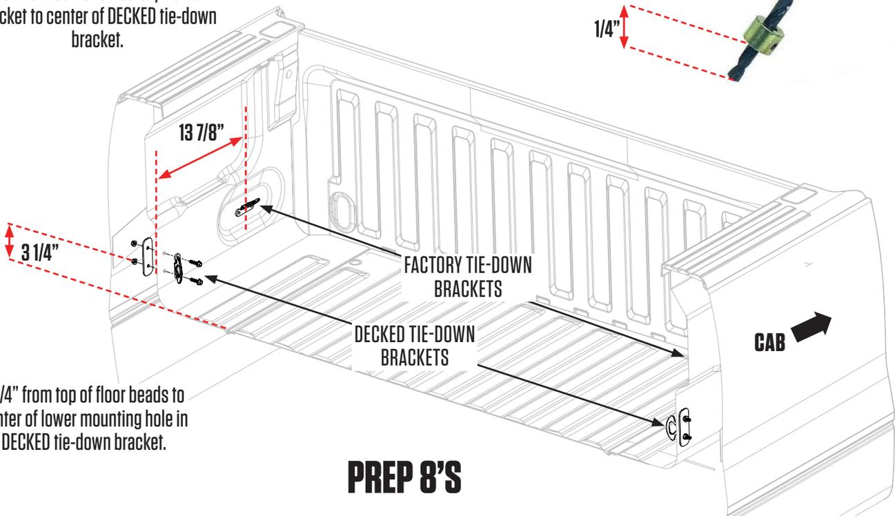
3 1/4" from top of floor beads to center of lower mounting hole in DECKED tie-down bracket.
