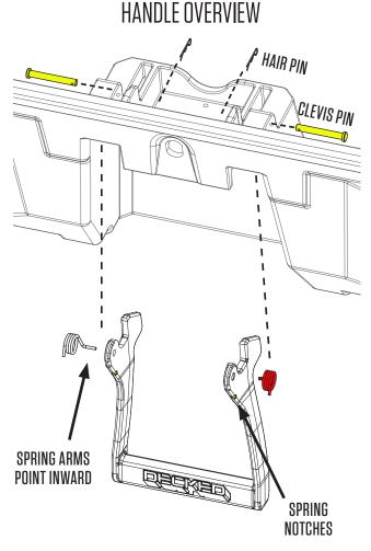
HELPFUL TIP: MAKE SURE SPRINGS HAVE THE LONG ARM HORIZONTAL AND SHORT LEG VERTICAL BEFORE INSERTING HANDLE
