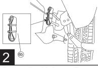
On some models that do not utilize this guide rubber tape is included. Wrap tape around bracket.
