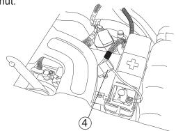
Attach ground lead to negative battery pole.
