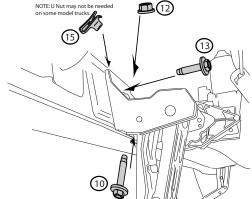
Set linkage into second to last sheetmetal tab / hole from rear. Use supplied bolt (10) and nut(12) to hold in position. Install bolt (13) into upper mounting hole and snug both bolts. Torque upper bolt (13) to 16ft-lbs(22N m) first and then torque lower bolt (10) and nut (12) to 16 ft-lb (22N m). Repeat linkage installation on Passenger side.
