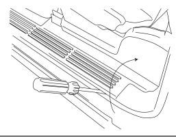
Pull up the carpet and thread both wires through the floor panel (same steps on passenger side EXCEPT drill 9/32" hole in metal and add rubber grommet).
