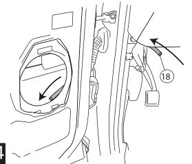
Feed longer wire of Step 13 through tube into door and pull out plastic tube on door side. Route wire along harness to switchplate.
