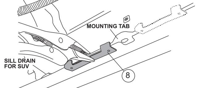
Clamp drill template to pinch weld about 1/8" behind the forward most mounting tab.
