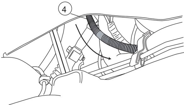
Poke hole through rubber grommet near front door on underside of floor panel with small phillips screwdriver. Push both wires through hole. (See Step 20 for passenger side notes.)
