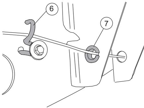
HD - Long Bed: Install plastic brake cable guide in forward hole of rear body mount.
