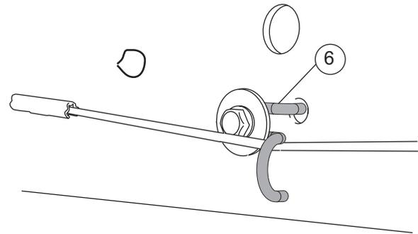
**2** Install replacement brake cable guides.
