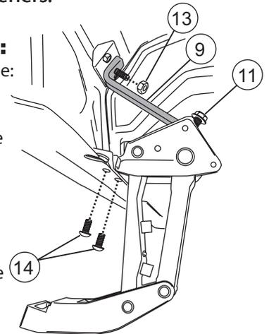
**10** Tighten button head fasteners and upper nut to 10 ft-lbs. Align the end of the board with the rear edge of the back door.
