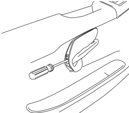
NOTE: Remove door light while removing door panel.
