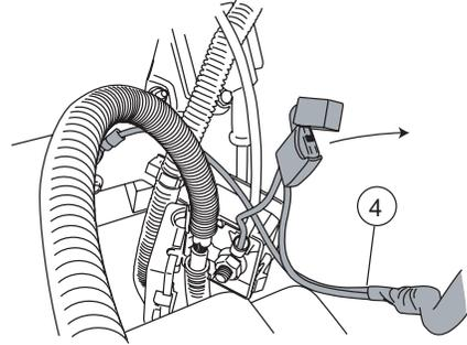
Attach ground lead to junction box mounting bracket. (See Step 15 for Diesel Engine grounding location)
