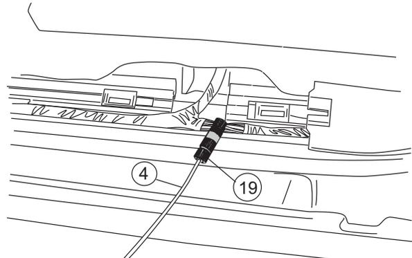
**Note: Crew Cab and SUV's only; these wires not used for Extended Cabs, Cut and tape off.**
