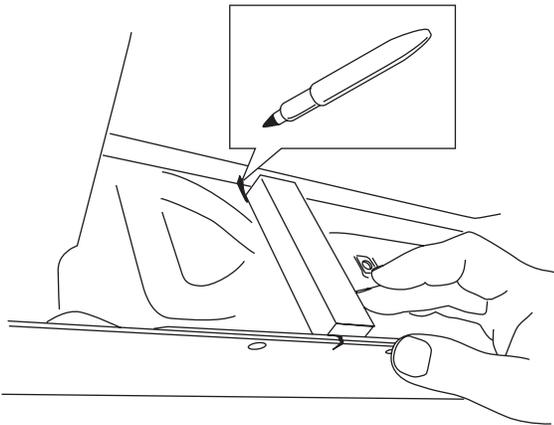
**7** Use a straight edge to make a vertical line centered between drilled mounting holes.
