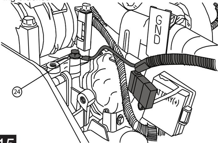
Route long end of wire harness above engine and down through passenger side wheel well. Zip tie harness to cowling clips on fire wall. Route short end down drivers side.
