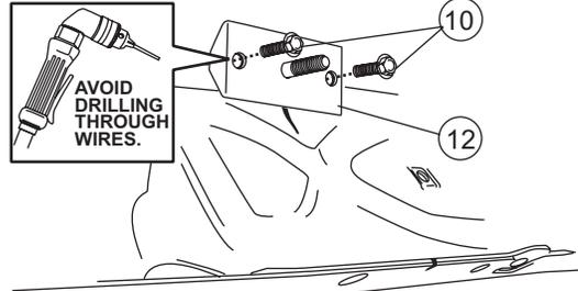
**8** File down any exposed screw tips from inside and cover with silicone.
