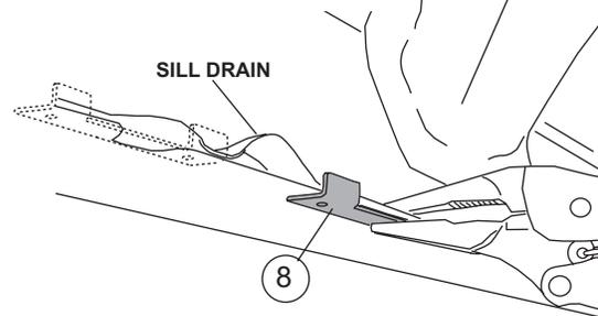
Clamp drill template about 1/16" forward of the rearmost sill drain.
