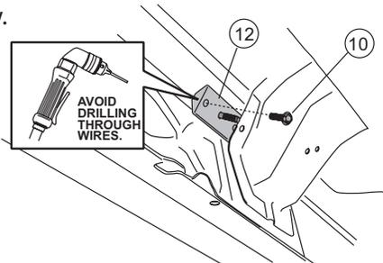
**9** File down any exposed screw tips from inside and cover with silicone.
