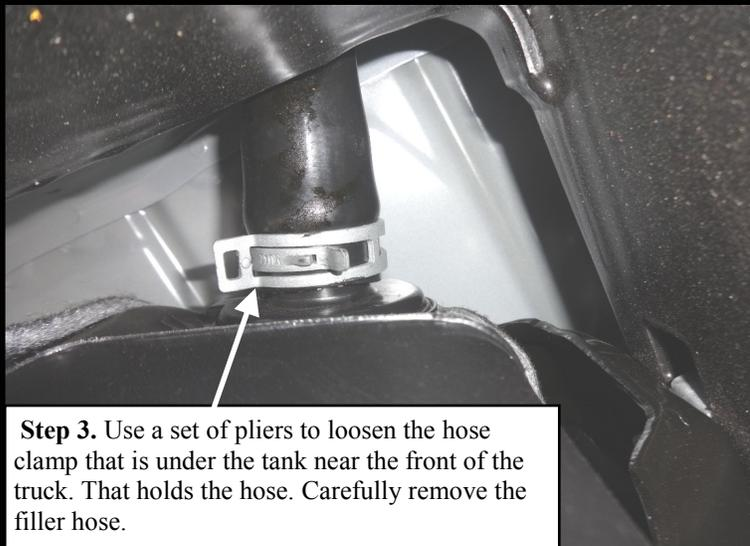
**Step 3.** Use a set of pliers to loosen the hose clamp that is under the tank near the front of the truck. That holds the hose. Carefully remove the filler hose.
