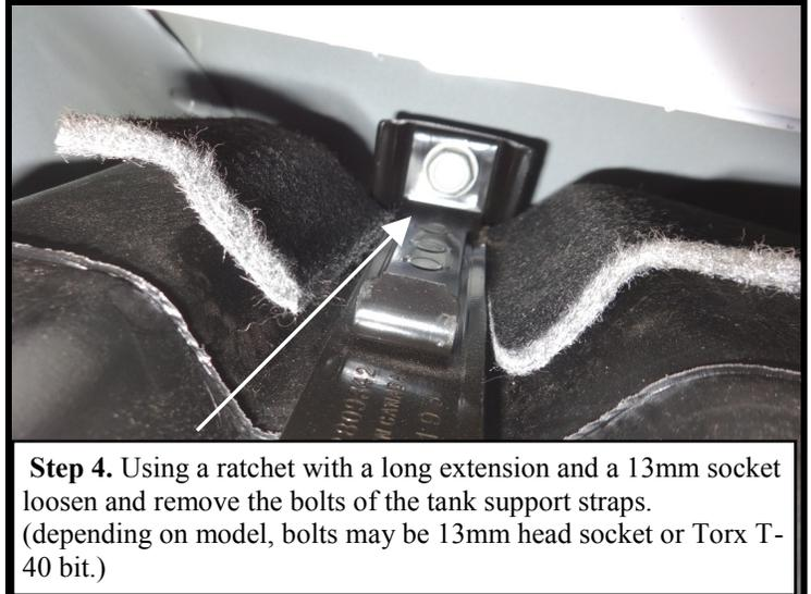
**Step 4.** Using a ratchet with a long extension and a 13mm socket loosen and remove the bolts of the tank support straps. (depending on model, bolts may be 13mm head socket or Torx T-40 bit.)
