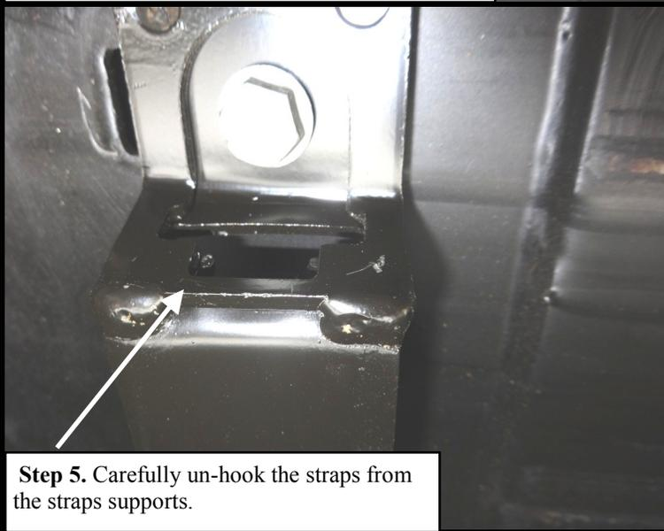
**Step 5.** Carefully un-hook the straps from the straps supports.
