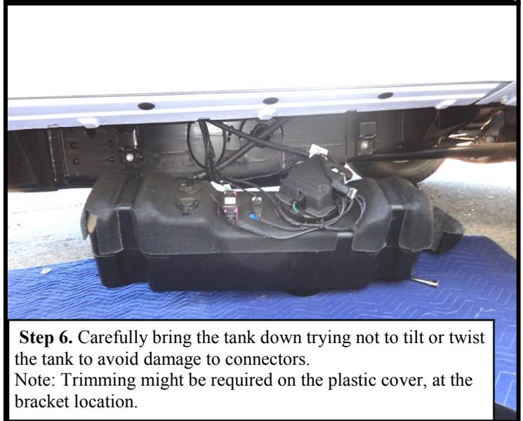
**Step 6.** Carefully bring the tank down trying not to tilt or twist the tank to avoid damage to connectors.
