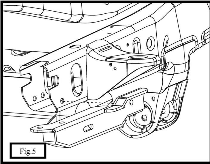
TO PROPERLY INSTALL BRACKETS YOU MUST DRILL HOLES TO THE FRAME. IN ORDER TO DO SO YOU MUST ALIGN THE BRACKETS TO THE FRAME USING THE EXISTING MOUNTING HOLES. AS SHOWN ON (FIG. 5)
