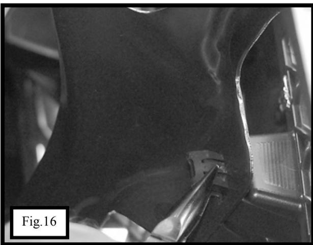
OPEN THE HOOD AND REMOVE THE RADIATOR COVER TO ACCESS THE FACTORY GRILLE SHELL. USING A SMALL FLAT HEAD SCREWDRIVER, REMOVE THE RETAINER PLUGS. USE A 10mm SOCKET TO REMOVE THE TWO OUTER BOLTS FROM THE GRILLE SHELL.
