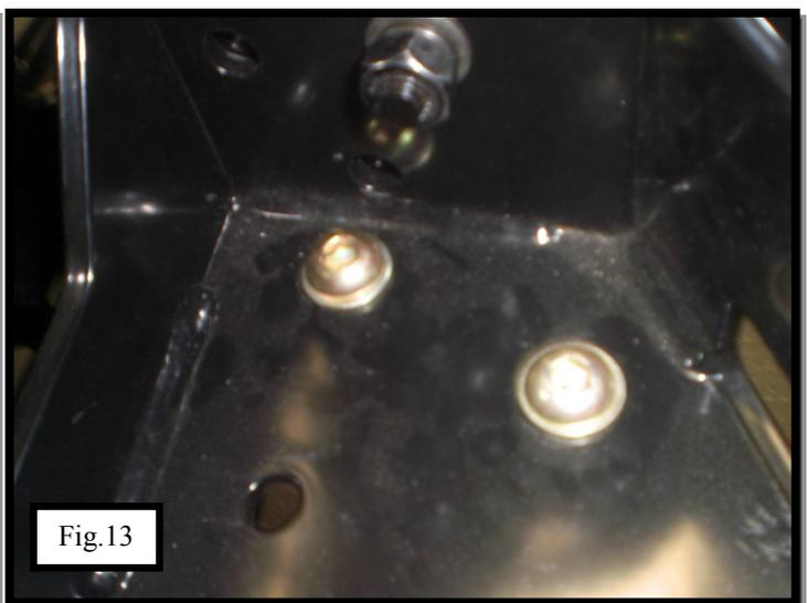
TO ATTACH WINCH TRAY USE (4) M12 BUTTON HEAD BOLTS, (8) M12 FLAT WASHERS, (4) M12 LOCK WASHERS, & (4) M12 HEX NUTS. YOU MAY NOW ALIGN AND ADJUST MOUNTING BRACKETS AND WINCH TRAY.
