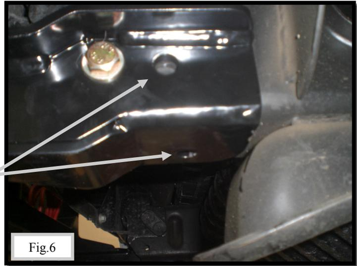
PLACE THE BRACKET ASIDE AND WITH A 1/4" DRILL BIT, DRILL A PILOT HOLE THROUGH THE FRAME. VERIFY THAT THE HOLE IS IN THE CORRECT LOCATION BY PLACING THE BRACKET BACK ON THE INSTALLED POSITION, THEN OPEN THE PILOT HOLE BY DRILLING THROUGH USING 1/2" DRILL BIT. **NOTE: PASSENGER SIDE ONLY REQUIRES ONE HOLE TO BE DRILLED INTO THE FRAME.**
