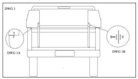
Step 3: On the underside of the tool box and close to the bed rail (rear of truck), drill a 5/16" hole to accept the "J" bolt. Push the "J" bolt thread up into the hole while hooking the bed rail lip. Your helper can then secure it with a fender washer, lock washer and 1/4" hex nut. See DWG 1A. Repeat at the front of the bed rail.
