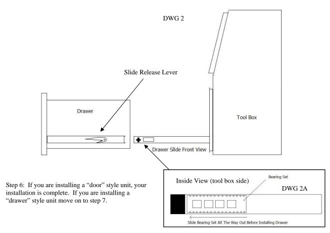
Step 7: When installing the drawer first be sure the drawer slide is in full extended position to accept the drawer. See DWG 2. IMPORTANT: be sure the bearing set on the drawer slide is also in the full outward position while sliding the drawer into place. Failure to do so will not allow drawer to lock into position.
