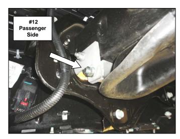
**Step-7** With assistance, position the RC2 Bull Bar up to the main brackets and attach the mounting flanges to the outside of each bracket using (2) 3/8" x 1" carriage bolts, (2) 3/8" flat washers, (2) 3/8" lock washers and (2) 3/8" hex nuts, (**Photo 13 & 14**).
