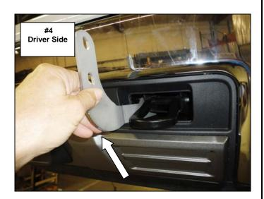
**Step-3** Hook the slot in the bracket over the shank of the front tow hook bolt, reinstall the front bolt nut and rear tow hook bolt to secure the bracket to the side of the frame, (**Photo 5**). Leave the nut and bolts loose for final adjustment.
