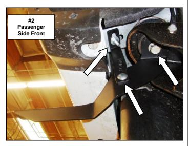
**Step-3** Remove the passenger side middle body mount bolt. Keep all existing bushing in place, and attach the passenger side middle bracket to the vehicle using the factory body mount bolt, (Photo 3 & 4). Leave the body mount bolt loose for final adjustment.
