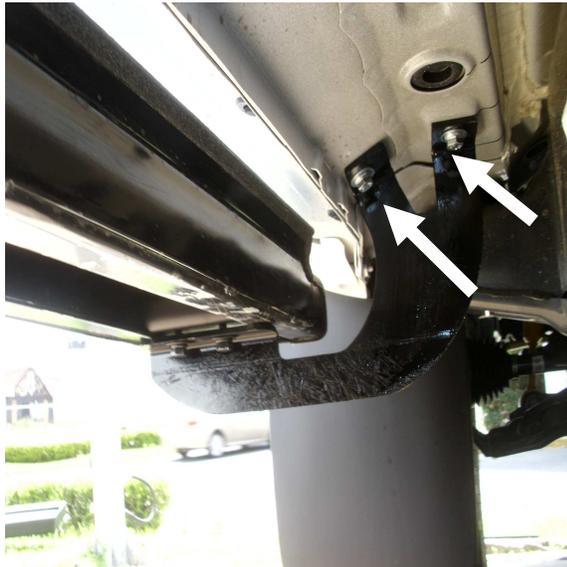
7. Place the sidebar on top of the mounting brackets. Position (3) of the U-brackets (included with the side step) inside the sidebar body, and align the U-brackets with the mounting brackets. Attach the side step and U-brackets to each mounting brackets using (2) 5/16" Hex head bolts, (2) 5/16" flat washers and (2) 5/16" lock washers. **ILLUSTRATION 1.**
