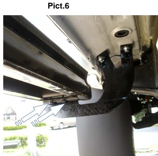
8. Align side bar RB10 and then tighten all bolts.
