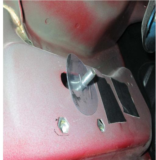
5. Place the front and middle bracket and attach to the bolt of the plate that was placed in the panel of the vehicle with: 3/8" flat and lock washers, 3/8" hex nut secure.
