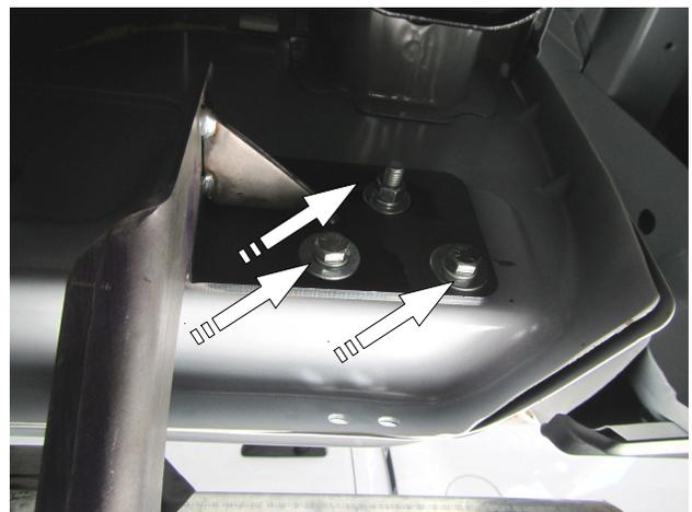
7. Place the sidebar on top of the mounting brackets. Position (3) of the U-brackets (included with the side step) inside the sidebar body, and align the U-brackets with the mounting brackets. Attach the side step and U-brackets to each mounting brackets using (2) 5/16" Hex head bolts, (2) 5/16" flat washers and (2) 5/16" lock washers. **ILLUSTRATION 3.**
