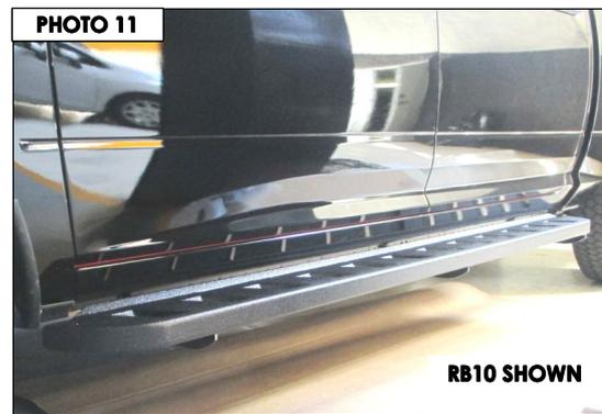
**11.** Align the running board with the vehicle and tighten all supplied nuts and bolts securing the running board and bracket assembly, **(Photo 11)**. Repeat the installation steps to install the passenger side brackets and running board. Remember to check and retighten all bolts periodically.
