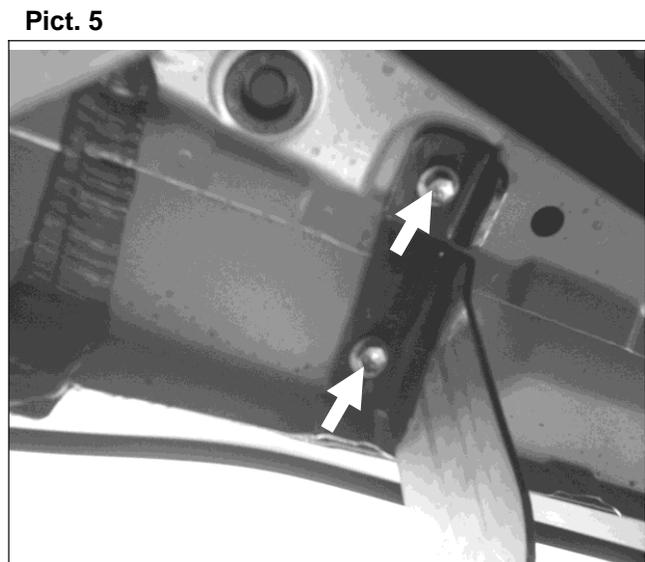
7. Place the sidebar on top of the mounting brackets. Position (3) of the U-brackets (included with the side step) inside the sidebar body, and align the U-brackets with the mounting brackets. Attach the side step and U-brackets to each mounting brackets using (2) 5/16" Hex head bolts, (2) 5/16" flat washers and (2) 5/16" lock washers. ILLUSTRATION 1.
