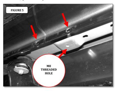
**Step-4** Attach the passenger side center bracket to the pinch mold using (2) 1/4" x 1" hex head bolts, (4) 1/4" flat washers, (2) 1/4" lock washers and (2) 1/4" hex nuts, and to the underside of the body using (1) M8 x 25mm hex bolt, (1) 5/16" lock washer and (1) 5/16" flat washer, (FIGURE 6 & 7).
