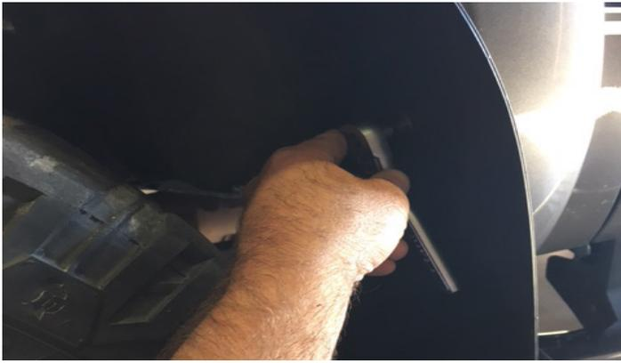
6. Fasten the flare to the truck with the factory fasteners. Check that the flare is parallel with the ground before tightening.
