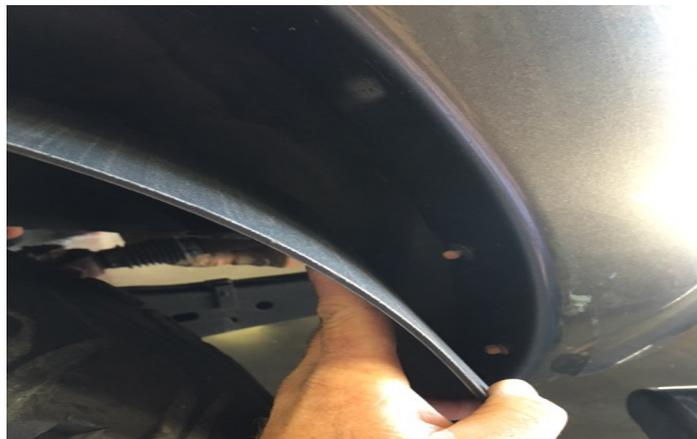
4. Align the mud flap so the bottom of the flare is parallel to the ground and at your desired height. Press the flare firmly against the fender to transfer the fastening locations.
