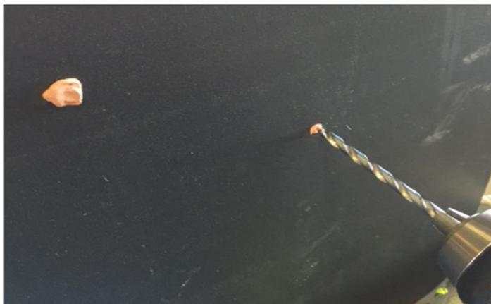
5. Drill fastening holes at the pre-marked locations in the mud flap to accommodate factory fastener size. If using supplies SS self drilling screws, drilling a small 1/8" pilot hole may help to ease installation.
