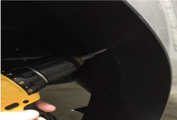
7. Install the SS self drilling screws at the other pre-drilled locations evenly around the flare.
