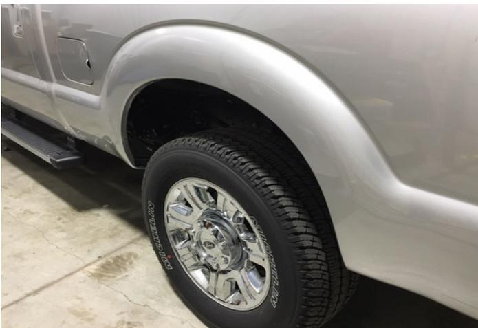
1. Clean the mounting location on your vehicle and check the location of factory fasteners and factory holes that can be used to fasten the flare. We recommend using the factory locations when possible then use the provided SS self tapping screws for further retention.
