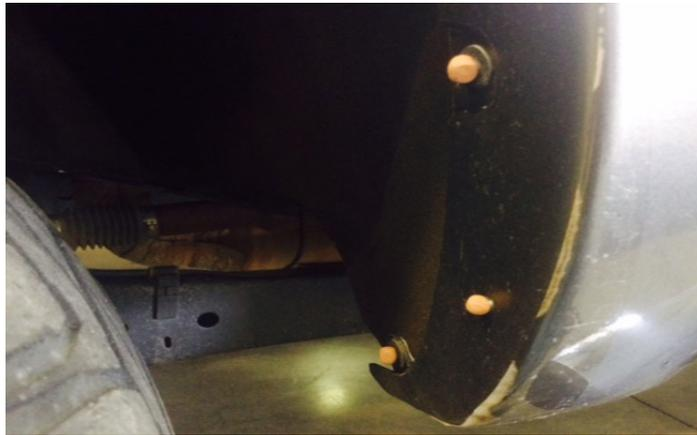
3. Transfer the factory hole locations to the flare mounting area. Mark the factory fasteners and other fastening locations with a small ball of clay or similar material.
