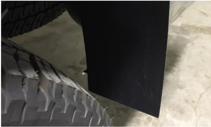
2. Align the flare on the fender lip for the amount of coverage and protection that is needed.
