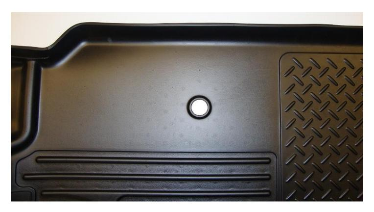
SHOWN TRIMMED FOR THE INSTALLATION OF THE JACK TOOL POUCH ON TOP OF THE LINER. TO TRIM, SIMPLY REMOVE THE MATERIAL FROM THE TOP OF THE RAISED BOSS AS SHOWN. A UTILITY KNIFE WORKS WELL FOR TRIMMING.
