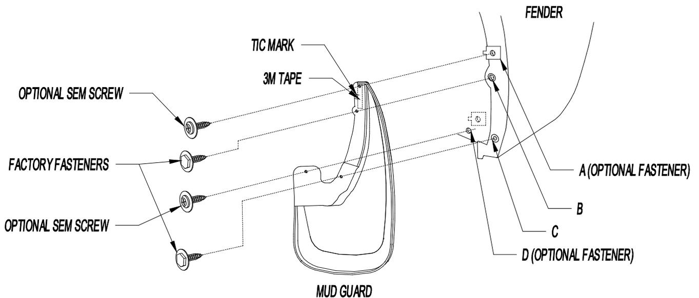
**NOTE: Turn wheels all the way left or right for easier installation. It may be necessary to remove the wheels before mud guard installation.**
