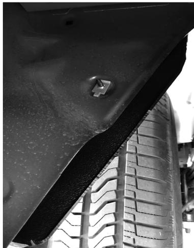
10. Align the 5 holes in the Wheel Well Guard with the factory screw locations and install the factory torx head screws. Install all screws before tightening.
