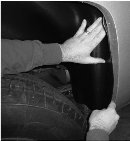
8. While working forward, tuck the liner behind the fenders inside edge.
