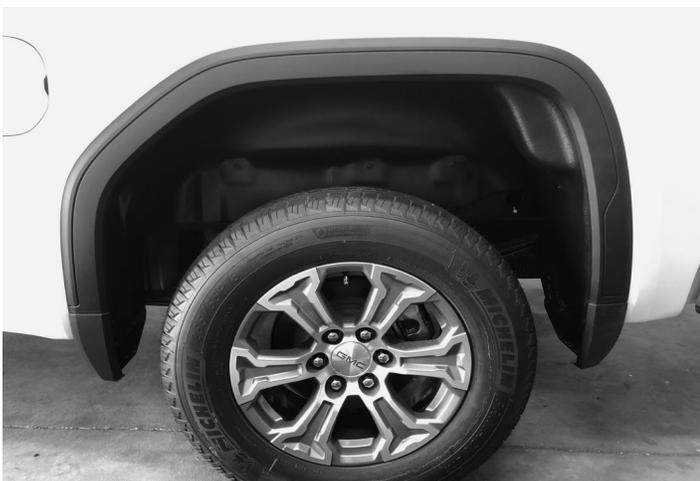
11. Once all fasteners at locations A,B,C, D, & E are installed, tighten with the Torx 10 bit / driver or phillips head screw driver if using supplied fasteners. Also tighten factory mud guard fasteners at this time.
