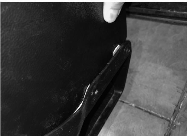
9. Tuck the front edge between the fender and factory mud guard.
