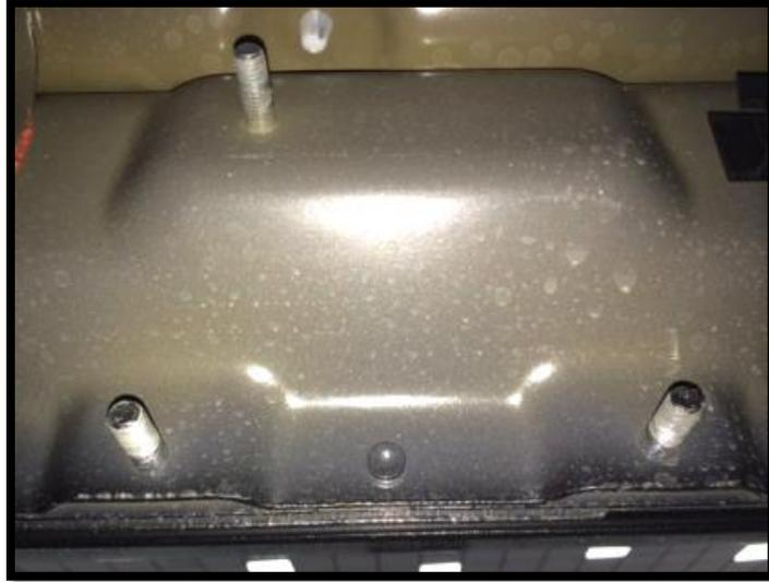
**Step 2:** Next, carefully raise the step assembly into position and align the three brackets with the nine 8mm OE threaded studs.
