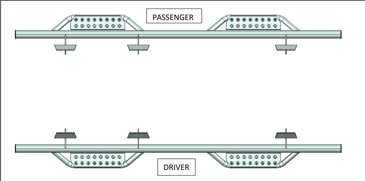
**Step 1:** Starting with the Driver Side. Remove all 8mm flange nuts from the 8mm factory threaded studs to remove the OE running boards.
