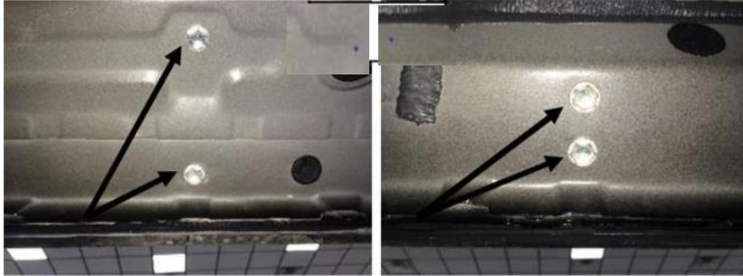
**Step 3:** Position step up to the body of the vehicle and align the brackets up with the factory mounting locations.
