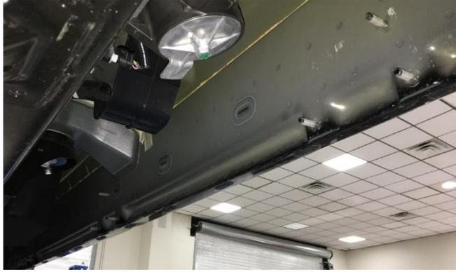
**Step 3:** On the inside rocker panel there will be three-attachment point consisting of three 8mm studs coming out from the panel. These studs may be covered in paint and will need to be cleaned before the installation.
