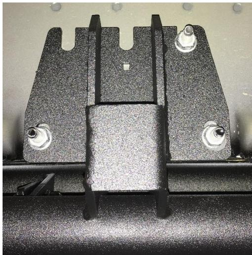
**Step 5:** Next, adjust the RAILS up snug and parallel with the cab of the vehicle and tighten all rocker panel brackets to 30 ft/Lbs. *DO NOT USE POWER TOOLS.*
