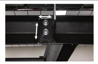
**Step 8:** After final positioning, start at the rear of the vehicle and tighten the lower portion of the bracket to 15-20 ft/lbs of torque. Continue this until all of the lower have been tighten then move to the top bolt and repeat the process.
