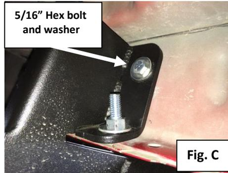
**Step 5.** Starting with the first bracket, fully tighten the bottom carriage bolts and continue with the center and rear bracket.
