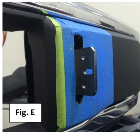
**Step 7:** Install Light bar/Pre-Runner to the bumper brackets using the supplied M6x20mm, M6 flange nuts and M6 washers and leave loose.
