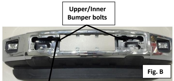
**Step 4:** Using a 3/8" drill bit, drill out the lower mounting hole through the bracket for Driver/Passenger. Secure with supplied 5/16"x1 1/2" hex bolt, 5/16" nuts and 5/16" washer.
