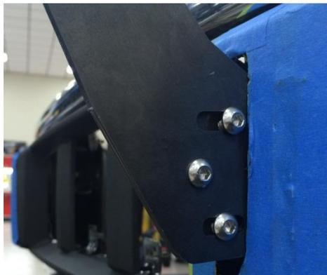
**Step 8:** After Light bar/Pre-runner has been properly adjusted, tighten all hardware. Your install is now complete.
