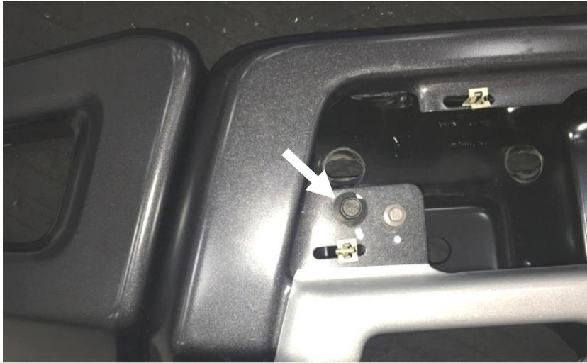
**Step 4:** Install the two mounting brackets Using the  $\frac{3}{4}$ " factory nut removed from **step 2** and the supplied  $\frac{1}{4}$ " x  $\frac{3}{4}$ " hex head flanged bolt and  $\frac{1}{4}$ " flanged nut. Tighten all hardware.
