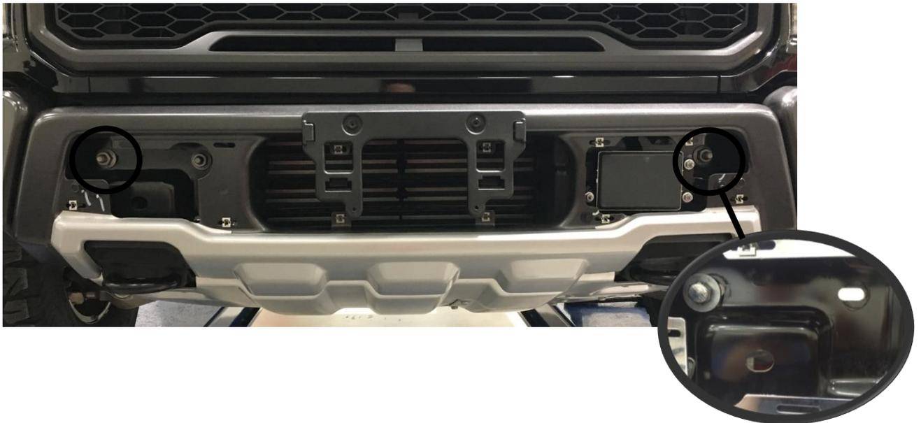
**Step 3:** Remove the outer bolt that attach the bumper end in the front. (Both sides)
