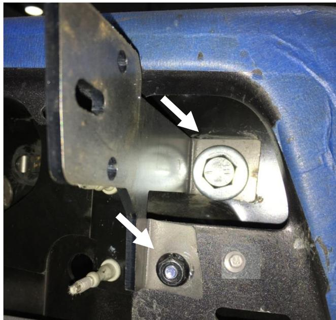
**Step 6:** Plastic bumper cover must be trimmed to expose mounting brackets. The measurements in this step are approximat. **NOTE: Take extra time and double check measurements before trimming the plastic.**
