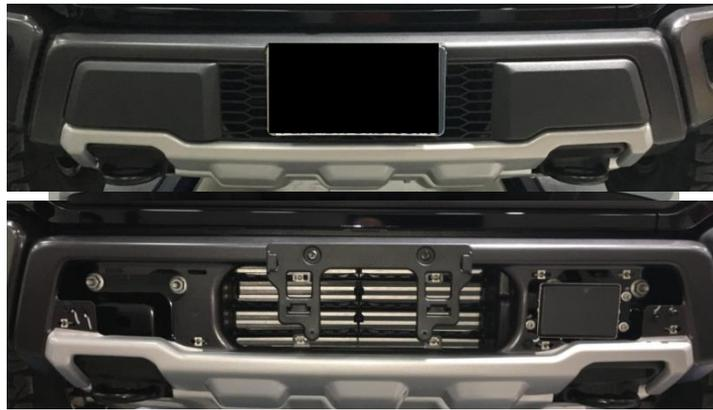
**Step 2:** Remove the outer nut that attaches the bumper to the frame (Both sides) .
