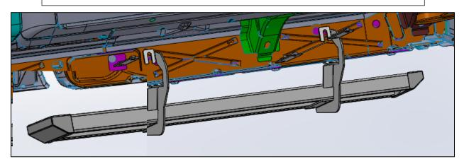
**Step 5:** Insert the supplied threaded brackets (x2) inside the running board lip over the top of each bracket.
