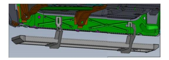
**Step 6:** Insert the supplied threaded brackets (x2) inside the running board lip over the top of each bracket.
