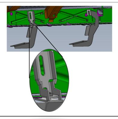
**Step 5:** Set running board along the top of all four brackets and center along the cab.
