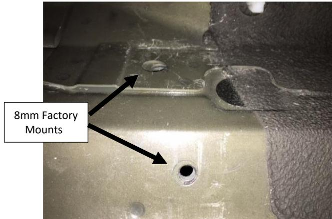
**Step 2:** Starting with the driver's side, install the (x2) rocker panel mounting brackets to the factory attachment points using the supplied M8X30mm Hex Cap Bolt with washer and leave loose at this time.
