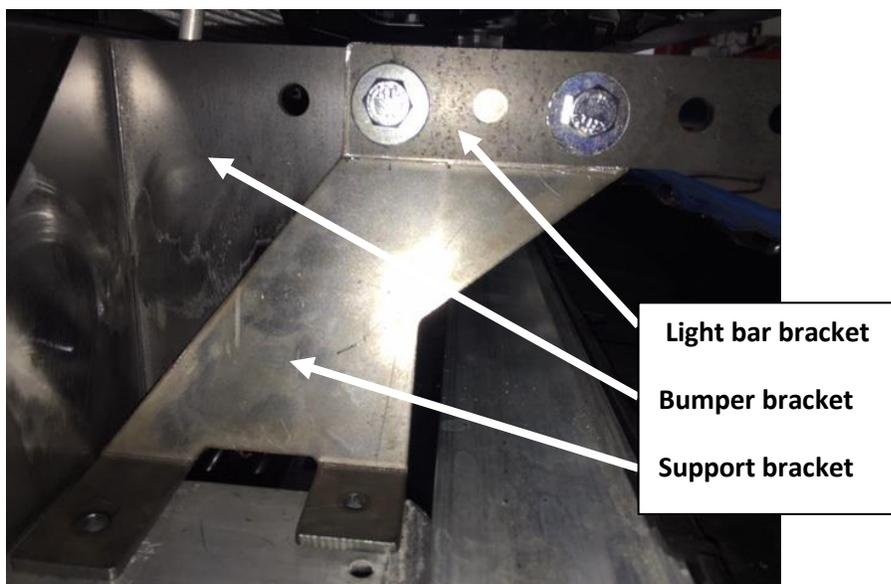
**Step 3:** Using the supplied ¼"x1" self tapping screws, secure Support bracket to the crash bar brace. (Both sides)
