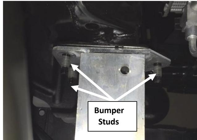
**Step 2:** Install the bumper bracket to the OE studs with the factory 12mm nuts and fully tighten to factory specs. (both sides)
