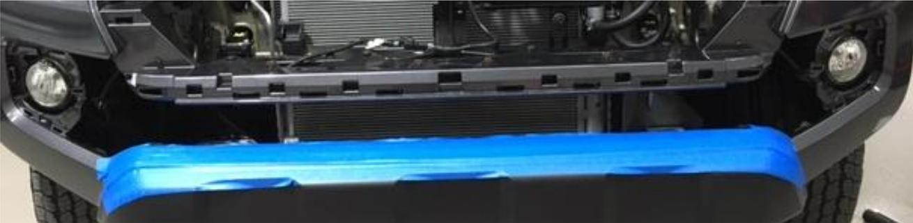
**Step 8:** Remove the plastic side cover by releasing the push pin and pulling forward from the clip. (both sides)
