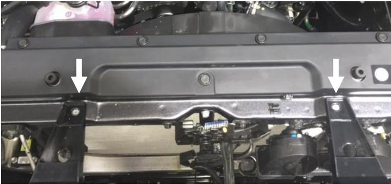
**Step 2:** Next remove the two push pins located on the left and right side of grill.
