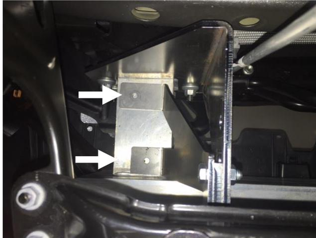
**Step 4:** After light bar is properly adjusted, tighten all hardware.
