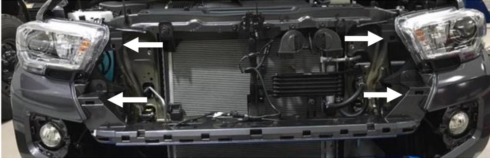
**Step 5:** Remove the plastic fog light trim piece by pulling forward to release the six pins (both sides)
