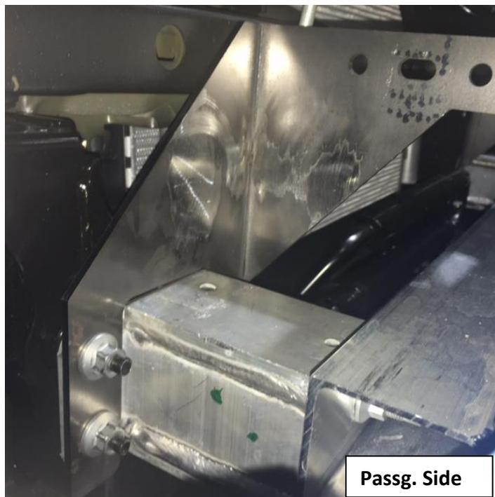
**Step 3:** Trim the ribs in the insert to clear the light bar brackets.
