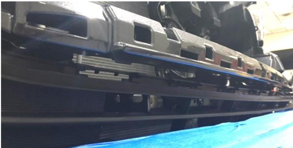
**Step 7:** Carefully push trim backwards through the core support to release from bumper and carefully pull out of the opening.
