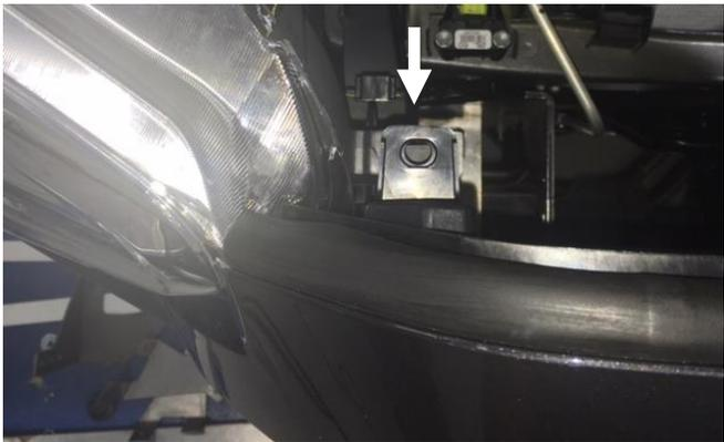
**Step 3:** Carefully left the two support brackets enough to clear the mounts.
