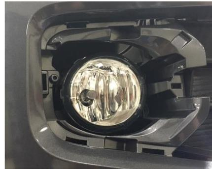
**Step 6:** Using a panel tool or flat head screw driver, release the 23 pins holding the plastic insert to the bumper.
