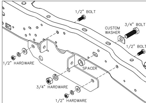
figure 7.2, exploded diagram of driver sideplate plate
