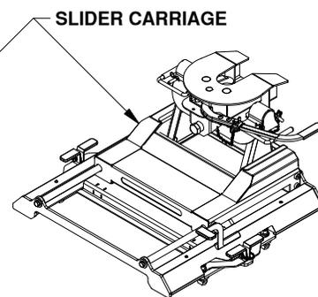
Figure H4: View of Slider Base with the Carriage in a back position. MANEUVERING POSITION
