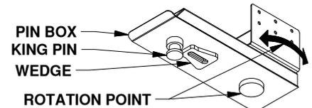
Figure F2: pin box with rotation point.
